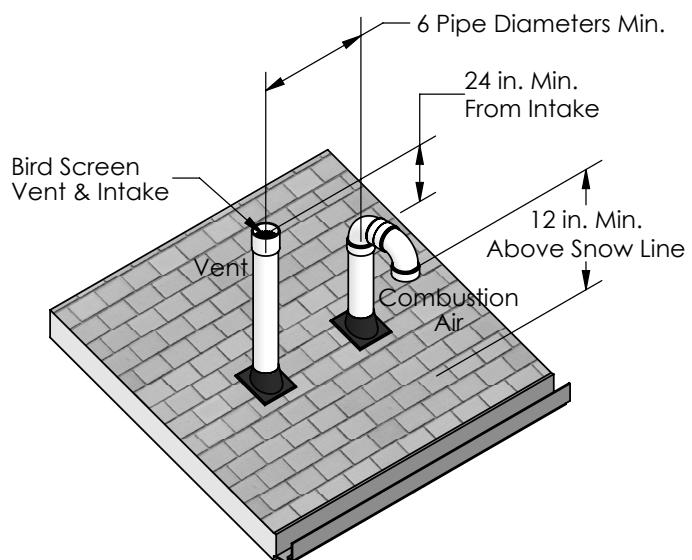
**Figure 13: Slopped Roof Termination**
