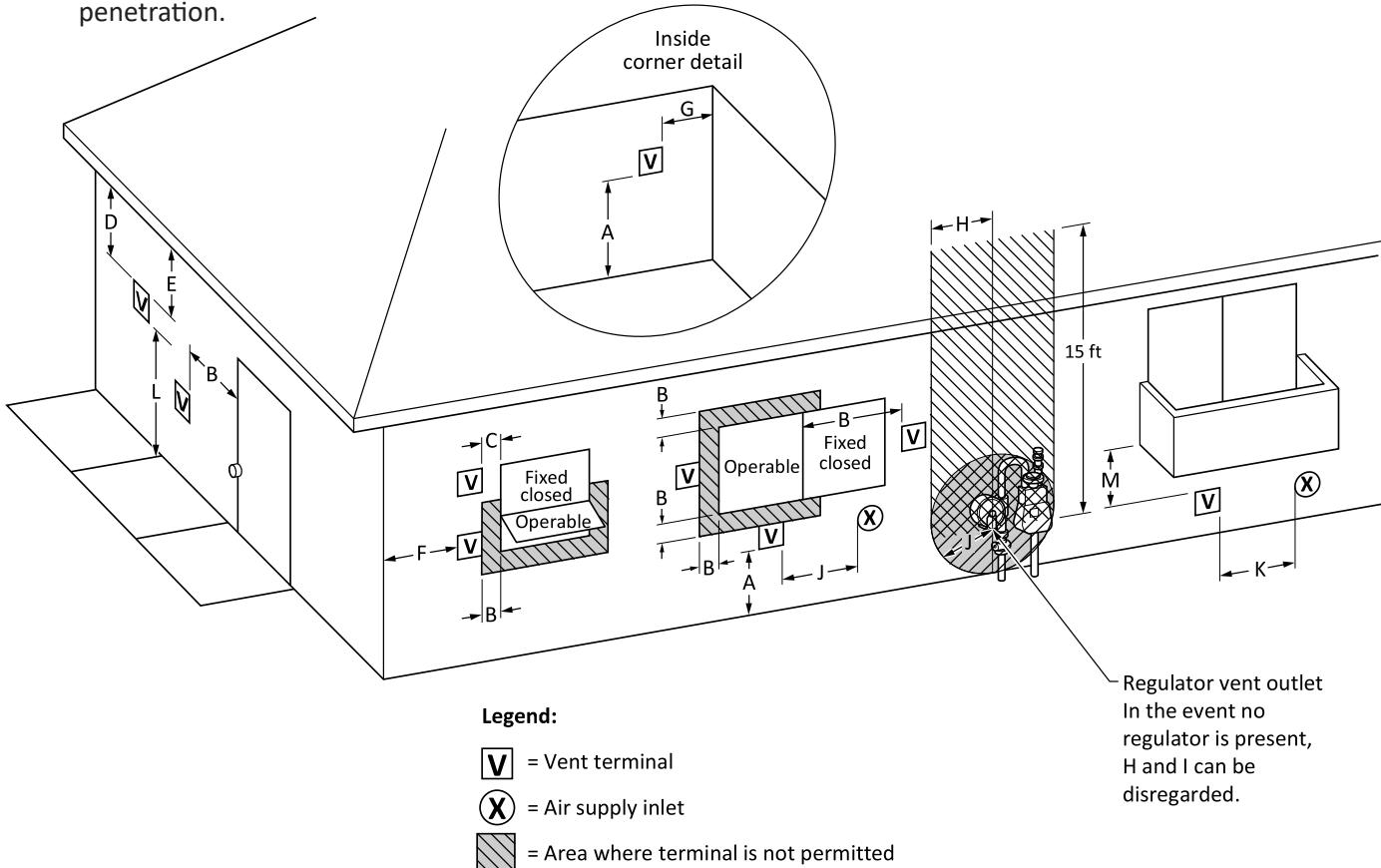
**Figure 11: Vent Terminal Clearances**
