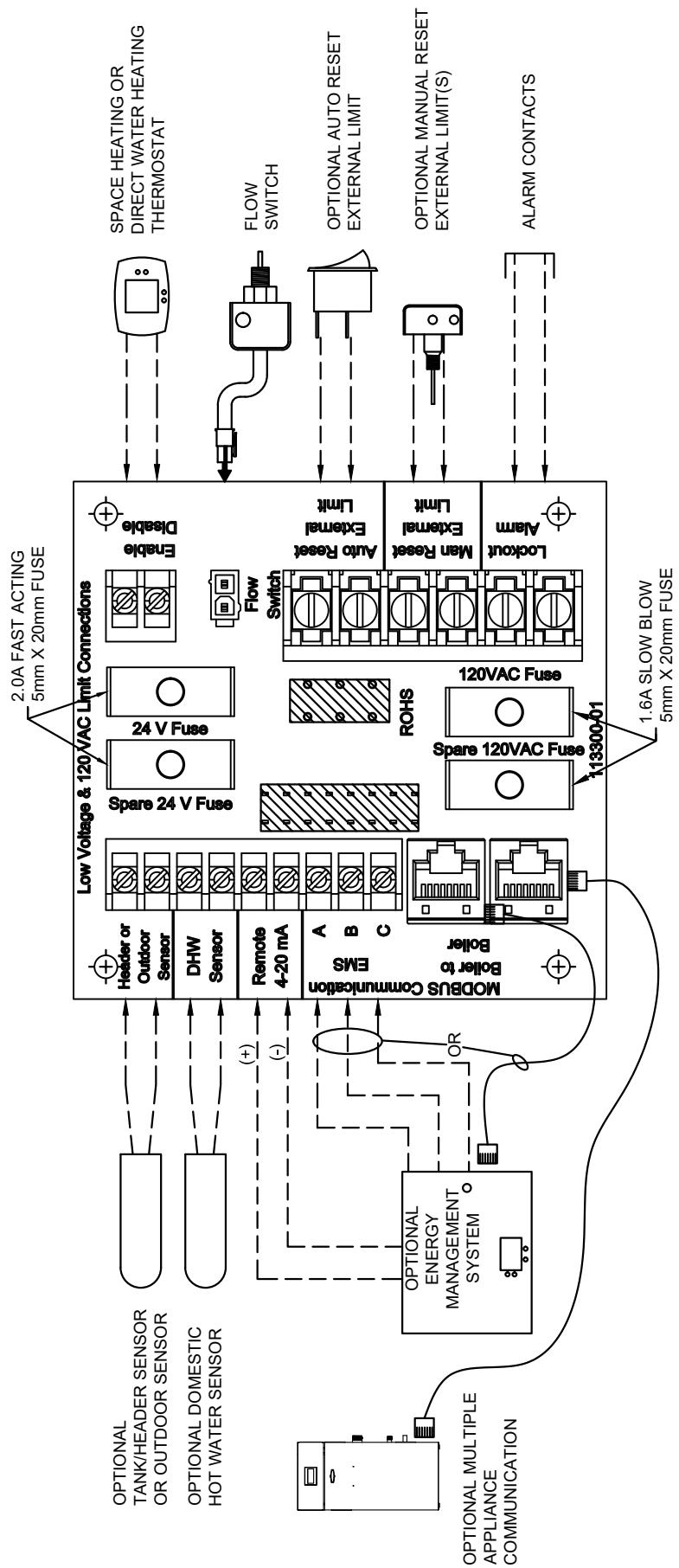
Figure 27: 1250-1500 Low Voltage and Limit Connections PCB
