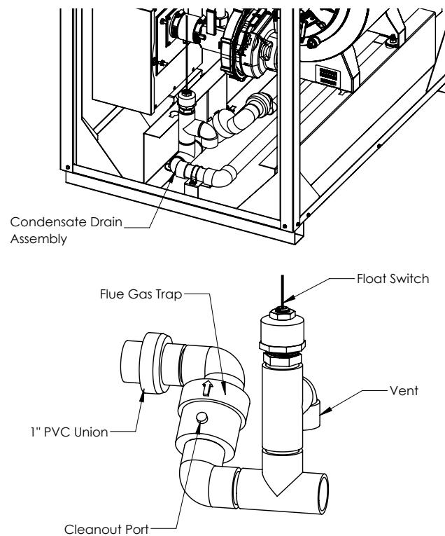
**Figure 17: Condensate Drain Assembly**
