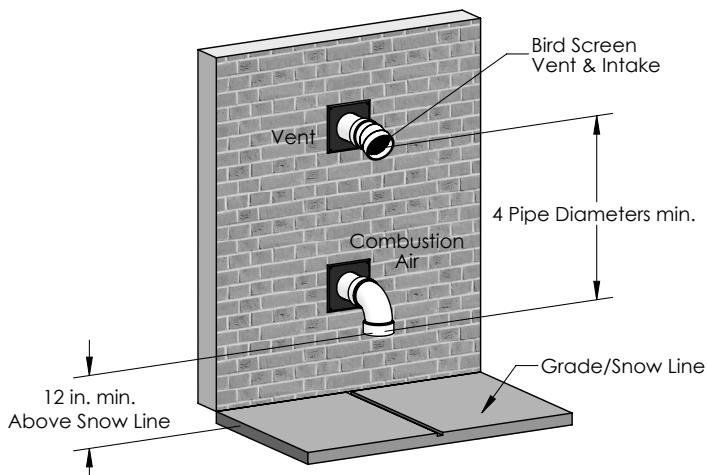
**Figure 12: Horizontal Sidewall Termination**
