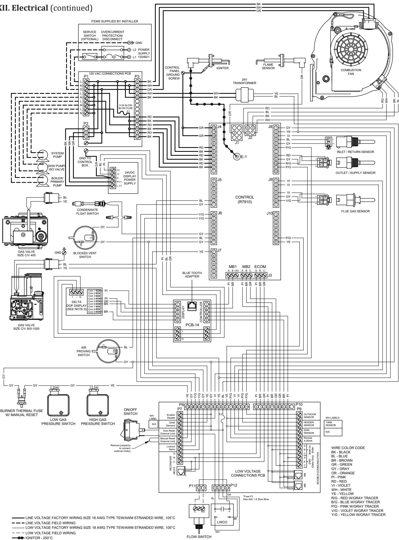
**Figure 28: 400-1000 Wire Schematic**
