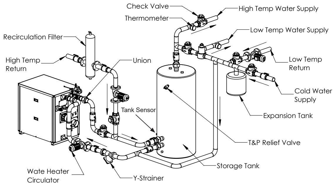
**Figure 19: Single Water Heater, Single Tank**
