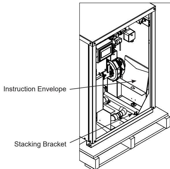
Figure 4: Loosely shipped parts locations
