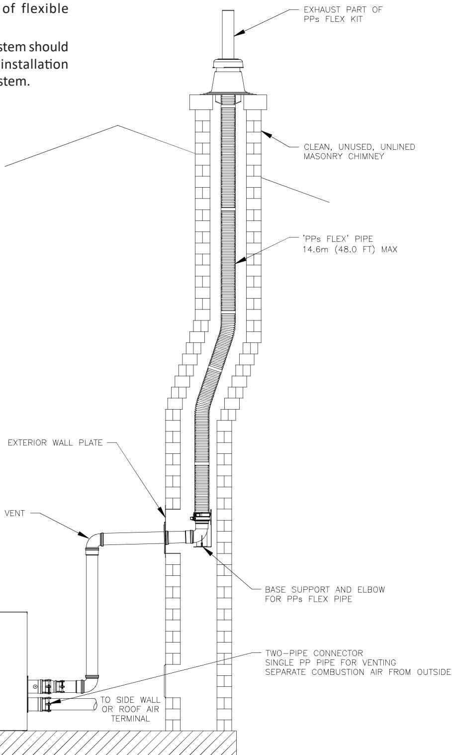
**Figure 16: Flexible Vent in Masonry Chimney with Separate Combustion Air Intake**
